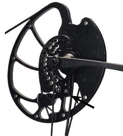
Each cam module needs to touch string to be in sync
